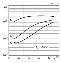
Switching Times Inductive Load Versus Temperature
